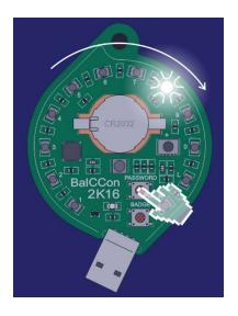
**SWITCH OFF:** The unit is automatically swithced OFF after it is disconnected from the USB port. You can also switch it OFF at any moment by pressing the lower button. A Rotating LED pattern in CCW direction signifies that the unit is OFF.
