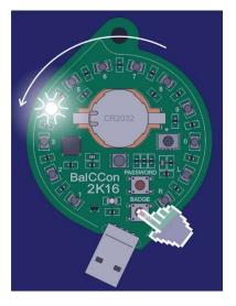
Password manager is the unit which generates, holds and types up to 10 independent passwords, each of them 15...20 characters long. Computer sees it as a standard USB HID keyboard, so it works with every computer which has a USB port, and requires no extra software installation. When you are asked to type the password, simply switch the unit ON, select the desired password and plug it in the USB port.
