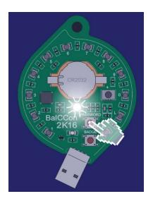
**SWITCH OFF:** The unit will automatically switch OFF after all of the TV codes have been transmitted. You can also switch the badge OFF at any moment by pressing the lower button. Rotating LED pattern in a CCW direction signifies that the unit is OFF.
