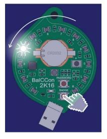
The unit starts transmitting infrared TV codes when the fast sequence on the central RGB led is finished, and the slow sequence runs.
