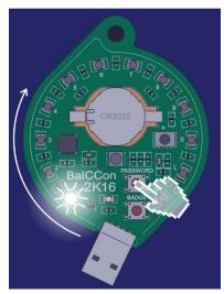
**Note:** USB stack is open-source assembler software, by **Bradley A. Minch**. In the BalcCCon Badge project, it was modified so that it accepts uppercase/lowercase charracters, servicing <shift> bit in USB packet.
